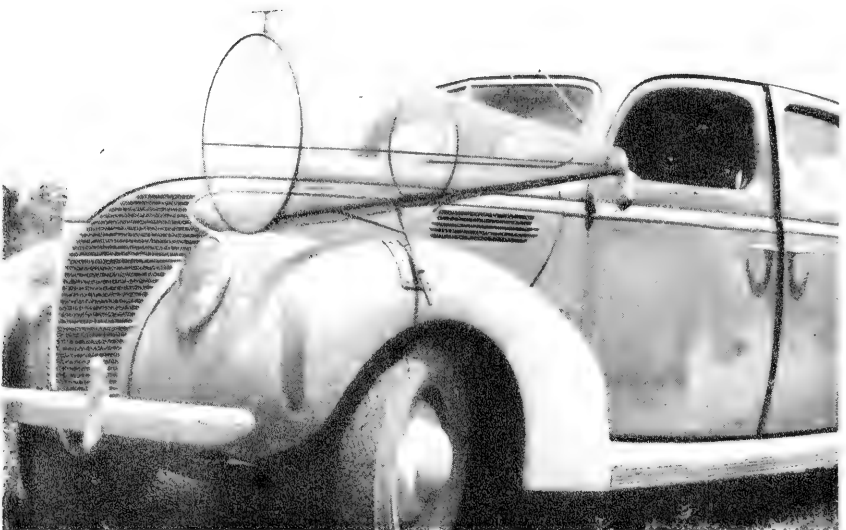
2. Cone trap mounted on the fender of an automobile as used in Moengo.
